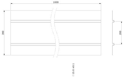
Dimensions for JGUFHSP165— All measurements in mm unless otherwise stated
