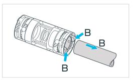
B – Push the collet down into the connector and pull the microduct away.
