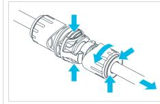
To release the pipe twist the locking cover 1/4 turn anti-clockwise, push the collet square against the face of the connector, then remove the pipe (cover misaligns with profile on body). Depress yellow catch to release gas block.
