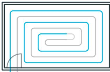
A spiral circuit pattern that achieves an even floor temperature with alternating flows and returns.
