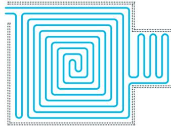
Serpentine and Counterflow pipe circuits can be combined in irregular shaped rooms.
