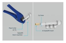
To cut and connect a stem ended manifold, firstly ensure the manifold stem is free of score marks. Cut the stem end square at the cut line indicated in the below diagram.
