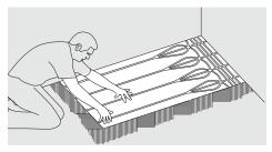
Press the first LowFit board firmly into the adhesive, applying even pressure to ensure the whole board is fully adhered to the floor below.
